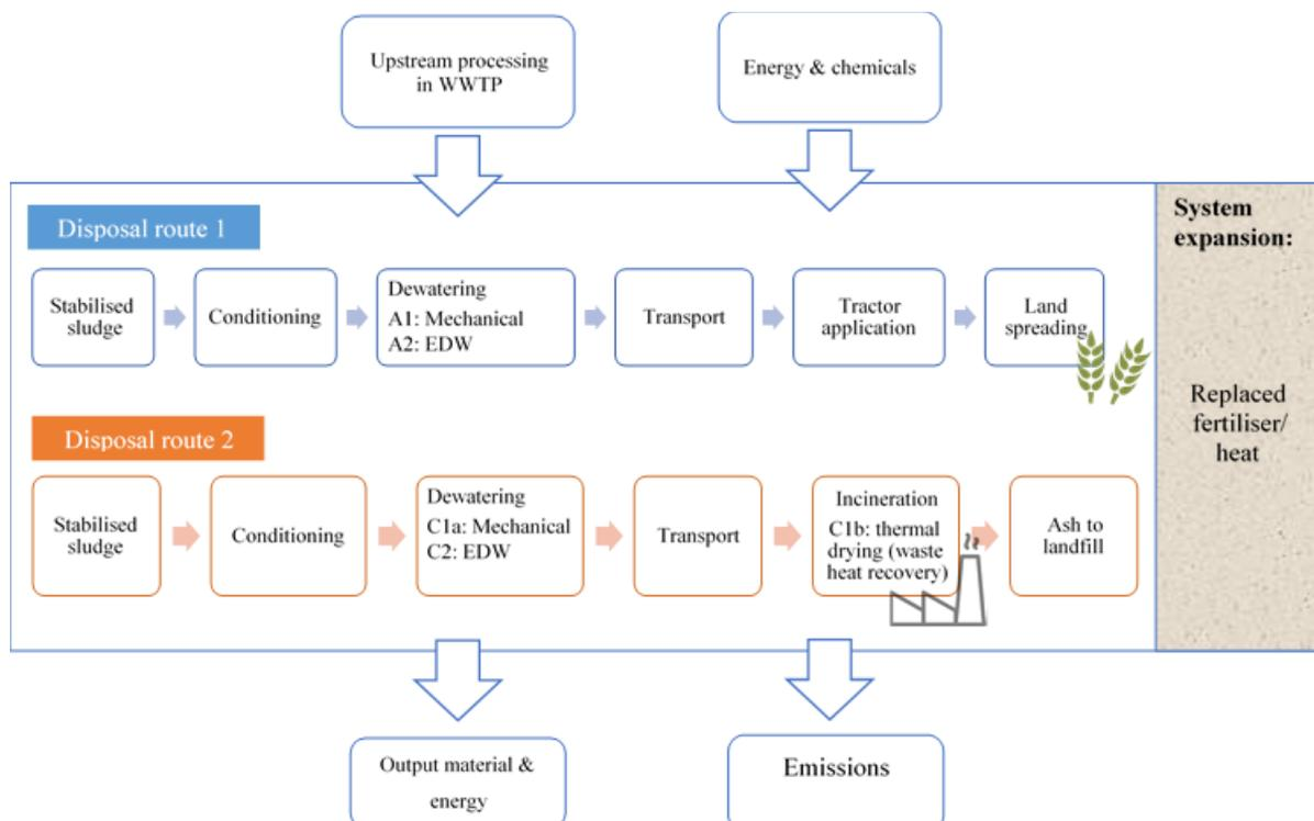
Figure 1 - Overview of system boundaries. Two sludge disposal routes were considered: land spreading (scenarios A1 & A2) and centralised incineration (scenarios C1 & C2). Since the sludge dewatering in C1 occurs in different locations, it is marked with C1a and C1b for clarity. EDW dewatering means the EDW unit is a retrofittable add-on module arranged after the existing mechanical dewatering facility.
